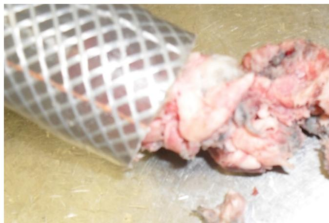
You must insure that the product you feed into the grinder is already small enough to pass through the sinew pipe. Sinew removal works well where you have a system with 3 plates and 2 knives as this ensures that the product is small enough to go through the sinew pipe and not block the hole.
