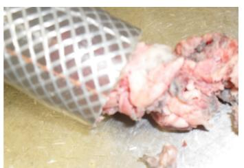
You must insure that the product you feed into the grinder is already small enough to pass through the sinew pipe. Sinew removal works well where you have a system with 3 plates and 2 knifes as this ensures that the product is small enough to go through the sinew pipe and not block the hole.
